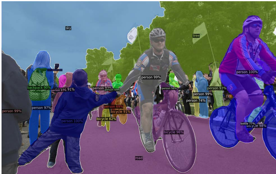
Figure 18: An example outcome of image detection using Mask-RCNN. Each detected object was given a label, put on a mask, and given the corresponding probability score. 26
