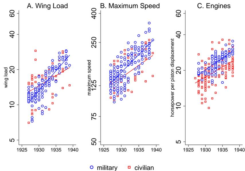
*Notes:* This figure shows the pace of technological progress in airframes measured using wing load (Panel A) and maximum speed (Panel B) and in engines measured using horsepower per piston displacement (Panel C) for the military and civilian markets.
