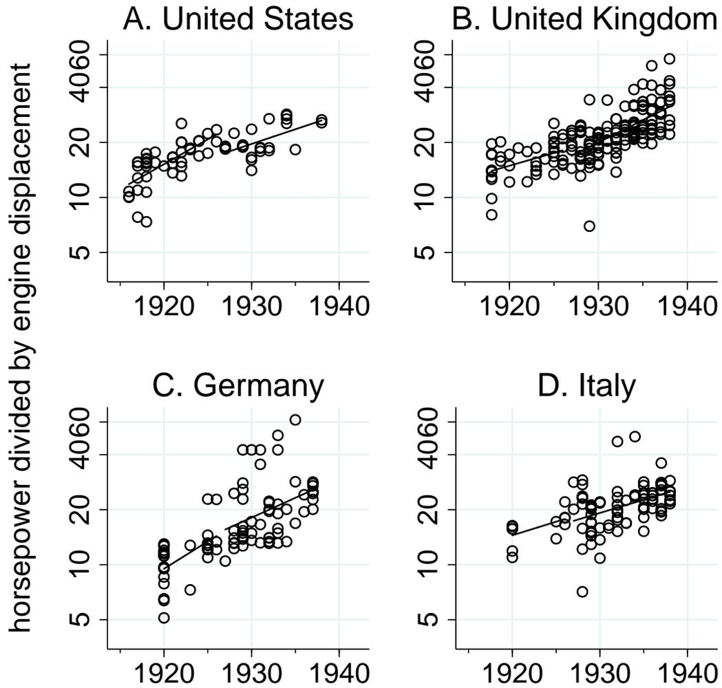
*Notes:* Each panel plots horsepower divided by piston displacement over time for the United States (Panel A), United Kingdom (Panel B), Germany (Panel C), and Italy (Panel D)
