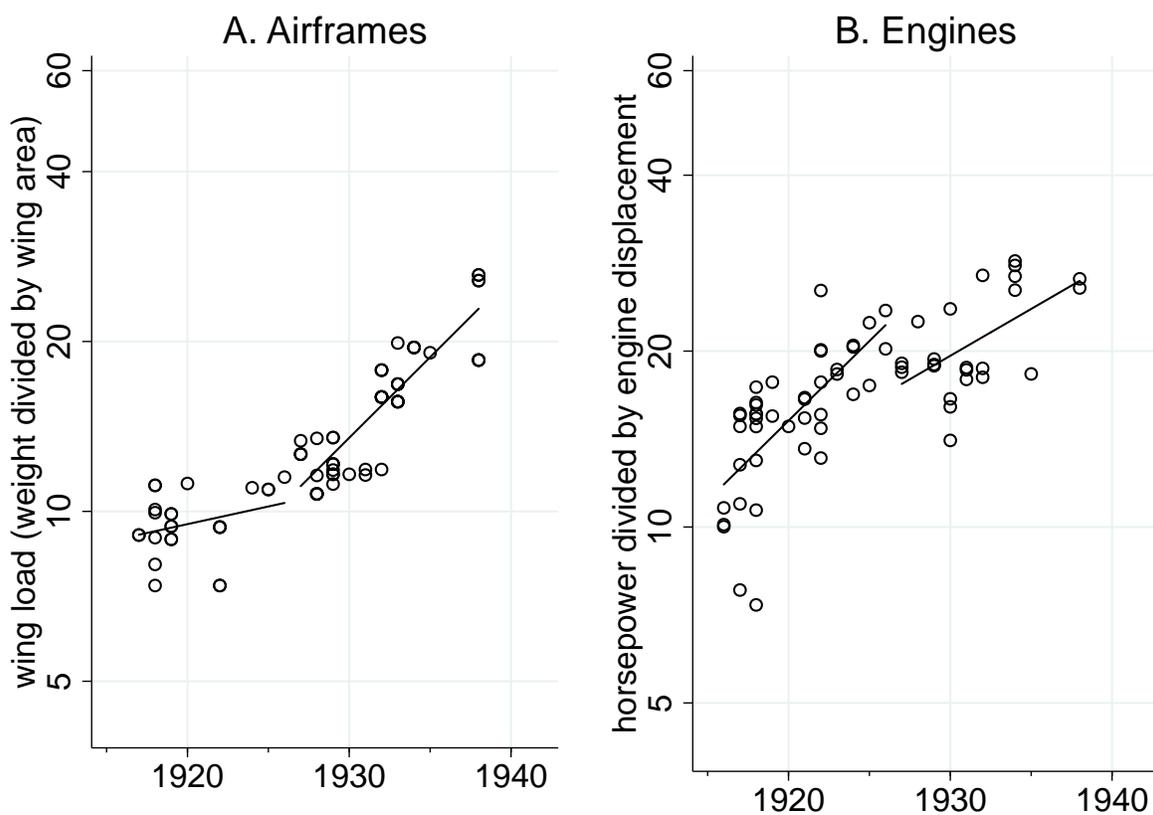
*Notes:* The figure shows innovation in military fighter airframes and aero engines for the United States between 1915 and 1938. Each dot plots gross weight divided by total wing area—i.e., wing load—of each fighter airframe (Panel A) and horsepower divided by engine displacement for each aero-engine (Panel B) introduced in a given year. The solid black lines in each panel reflect the best fit before and after 1926.
