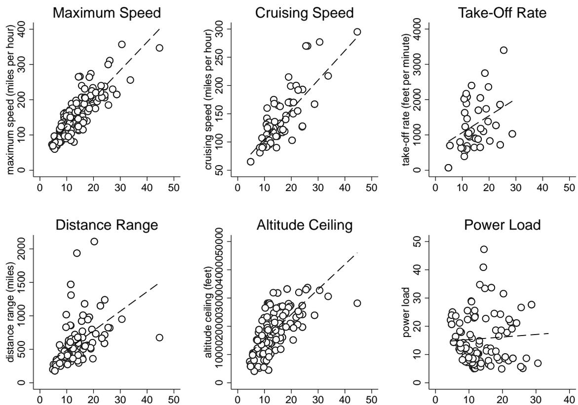
*Notes:* Each panel shows the relationship between wing load and the given alternative measure of airframe performance for the US airframe industry.
