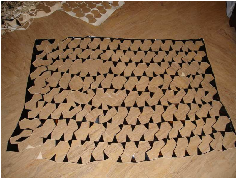
Figure 8: Laminated Rexine Wastage from Cutting Pentagons
