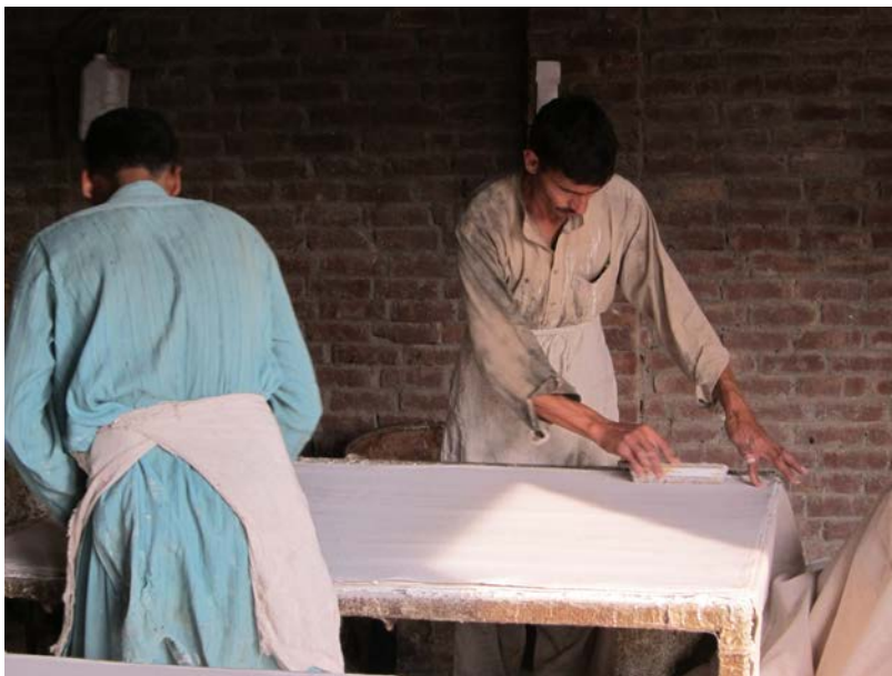
Figure 2: Making the Laminated Rexine Sheet (Step 1)
