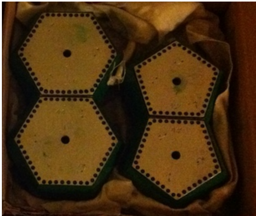
Figure 6: Traditional 2-Hexagon and 2-Pentagon Dies
