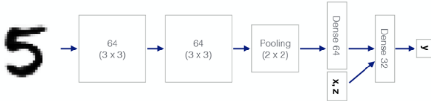
Figure 6: The network architecture used in Hartford et al. [13]. Variables \mathbf{x}, \mathbf{z} contain structured business information (e.g., product IDs and prices) that is mixed with images of handwritten digits in our network.
