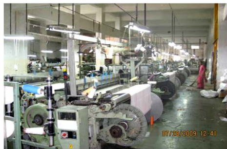
(3) Weaving the fabric on the weaving loom
