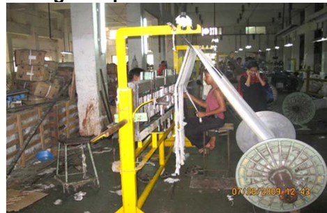
(2) Drawing the warp beam ready for weaving
