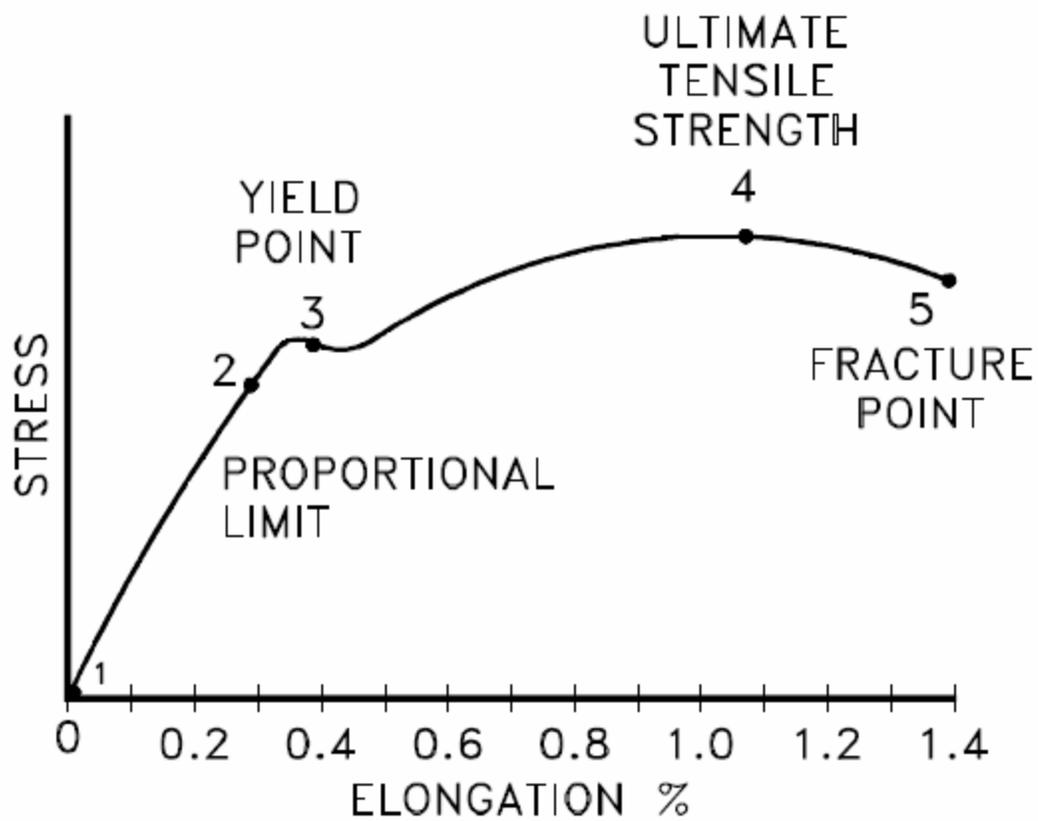
**Figure 7. Stress-strain curve for a typical ductile material**
