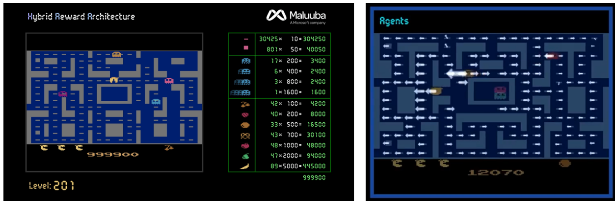
Figure 2: Screen-shots of the Maluuba system playing Ms Pac-Man. On the left, you see the game board. On the right, the authors have assigned arrows showing the current direction for Ms Pac-Man that is advised by different locations on the board, each corresponding to a distinct Deep Neural Network.
