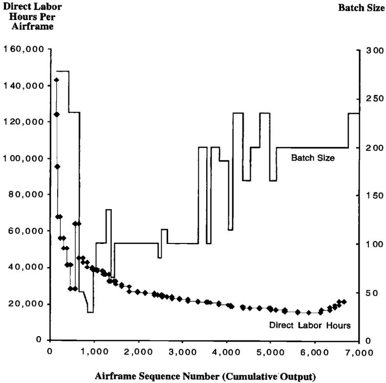
Fig. 4.9 The effect of batch size
